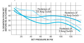
Deadband helps to prevent oscillation or "hunting". In other words, without sufficient deadband, the switch will be actuating and de-actuating too often. For applications where it is critical to de-actuate with less deadband, a 3 Amp switch is available. See specifications below.
